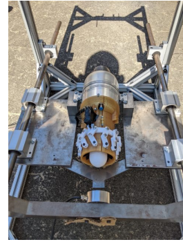
(b) VIGV system installed on the engine
